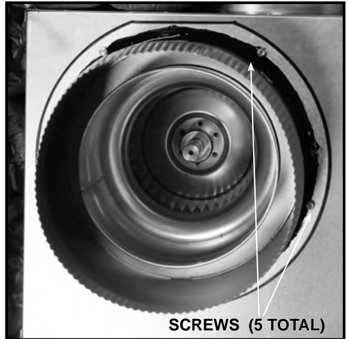
Figure 8.4 Base Plate Fastened to Intake
