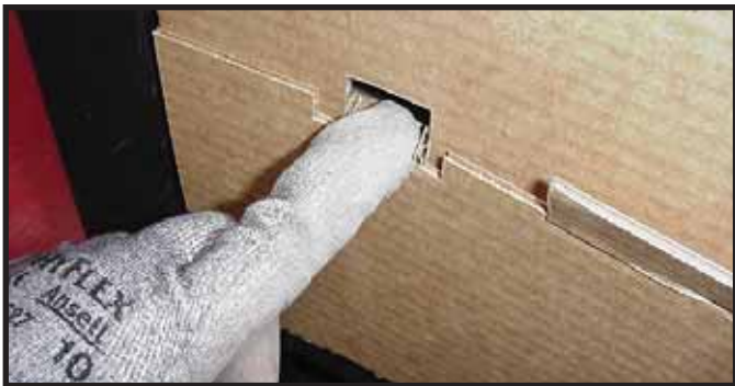
Figure 11.10 Securing Tabs Inside Front of Splatter Guard
