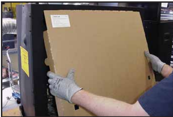
Figure 11.5 Installation of Splatter Guard
