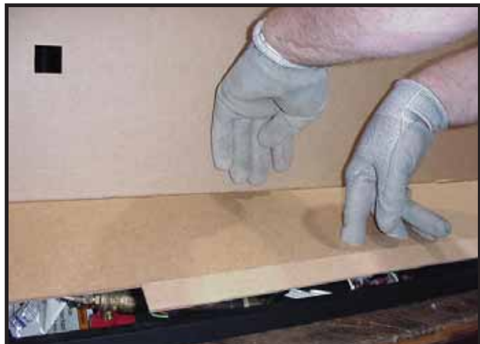
Figure 11.9 Opening Lower Access Panel
