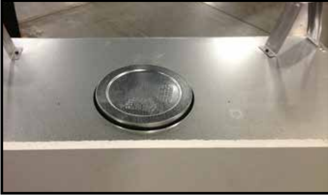
Figure 9.1 Seal Cap in Position
