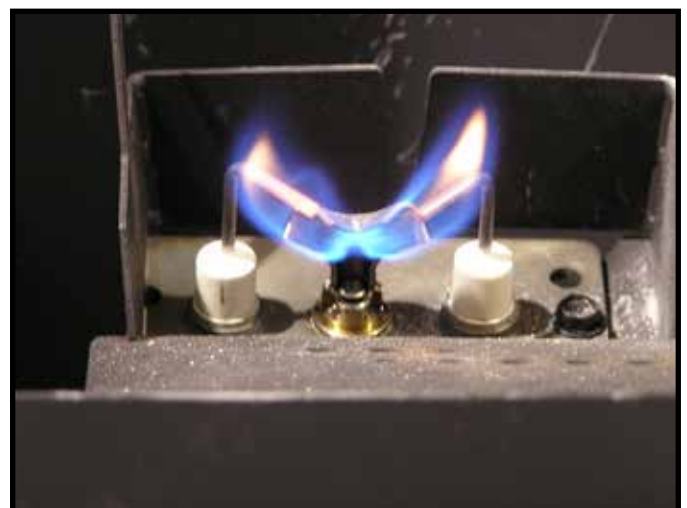
Figure 3.1 IPI Pilot Flame Patterns
