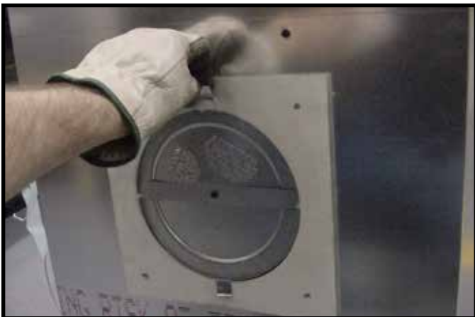
Figure 9.7 Fold the tabs toward the center of the seal cap (90°) and remove the insulation gasket.
