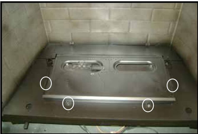
Figure 3.9 Remove Burner Skirt
