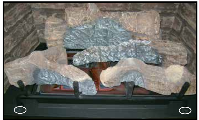
Figure 3.6 Remove Screws from Front Tab
