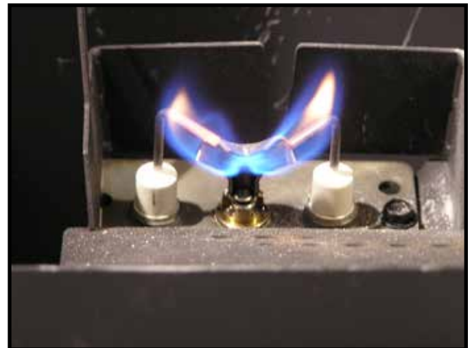
Figure 3.1 IPI Pilot Flame Patterns
