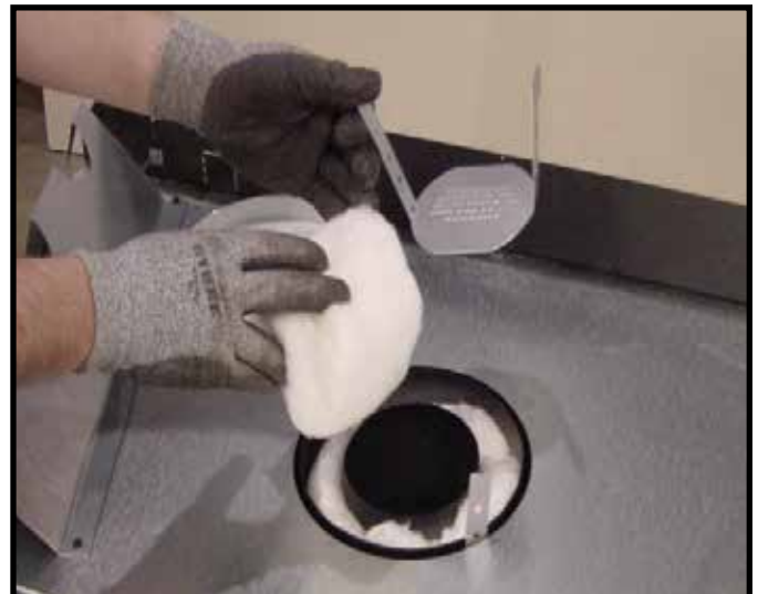
Figure 9.4 Remove the insulation basket and white insulation from the center vent pipe.
