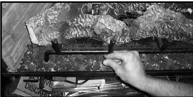
Figure 14.4 Placement of Vermiculite
