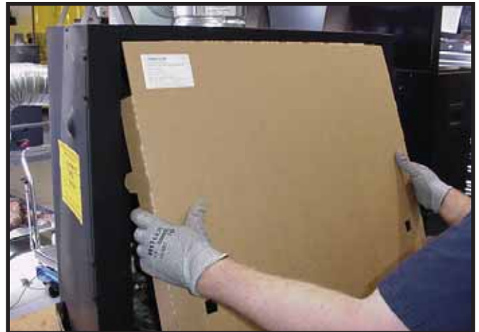
Figure 13.4 Installation of Splatter Guard
